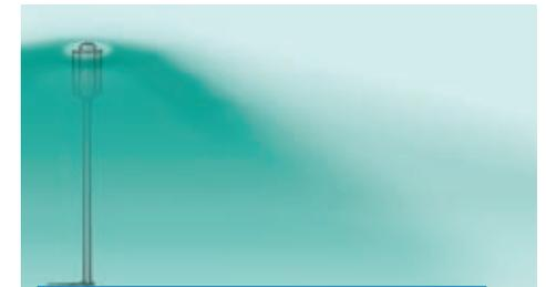
Within the overall distribution of radio waves from a base station across its cell, there is a zone where the concentration is higher than elsewhere.
